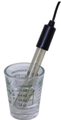
soaking, place the meter's electrode into CWP's Rejuve It!™ cleaning solution and brush very lightly with a soft tooth brush to remove unwanted minerals and organics from the glass bulb. If the meter still can't be calibrated the electrode's life may be over and a new electrode should be purchased. If it is within the warranty period please return the meter from where it was purchased or send it to CWP Instruments 9220 SE Stark Street Portland, Oregon 97216.
