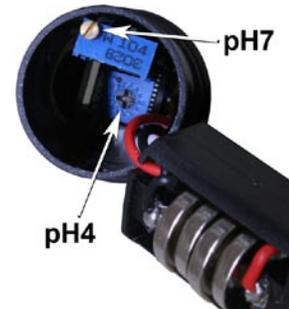
1. Turn the meter ON, remove the battery cap and pull the battery compartment out of the body. Let it hang to the side of the body. Place the meter's electrode into clean distilled water. Gently stir and then remove the meter from the water and blot the excess from the meter's body and glass electrode with a tissue.
